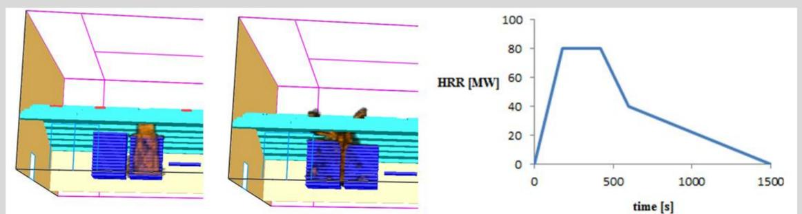
Figure: Results of the advanced model: gradual transfer of flames from the first burning panel across all panels in the paternoster (left), graph (smoothed) of the calculated HRR (right).
